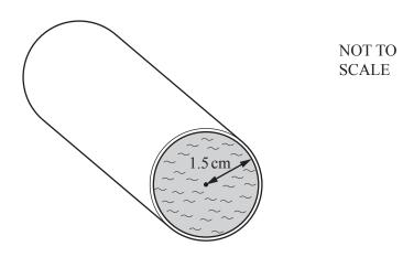
Water flows through a cylindrical pipe at a speed of 8 cm/s. The radius of the circular cross-section is 1.5 cm and the pipe is always completely full of water.
